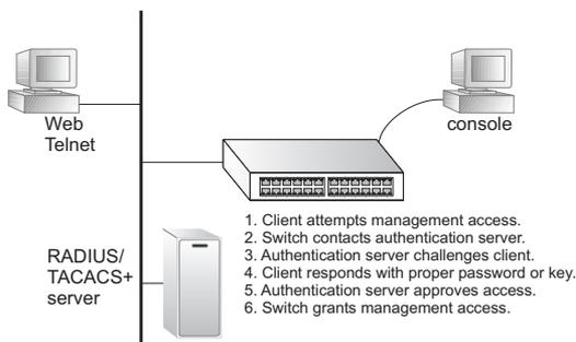
RADIUS uses UDP while TACACS+ uses TCP. UDP only offers best effort delivery, while TCP offers a connection-oriented transport. Also, note that RADIUS encrypts only the password in the access-request packet from the client to the server, while TACACS+ encrypts the entire body of the packet.
